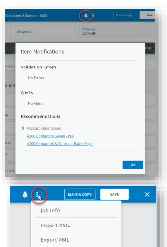
When you click **Bell icon** or when you save your configuration, the system will check for Validation Errors and Alerts and will display the Technical Data Sheet for Contactors and Starters.
